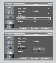
If no signal is being received or the signal is very weak, a blue screen automatically replaces the noisy picture background.
